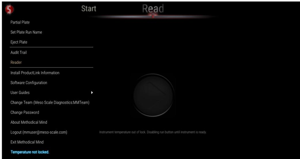
**FIGURE 4.1.** Methodical Mind indicating an error condition.
