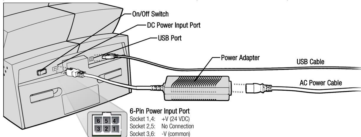
FIGURE 3.1. MESO QuickPlex Q 60MM I/O panel and connections
